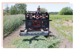
**Photo 2.** The crimper Ryan made using a disassembled crimper from an old haybine that they modified to fit onto the pallet forks of a tractor. For a full video of the crimper in action, visit: <u>efao.ca/no-till-fall-broccoli-2020</u>.
